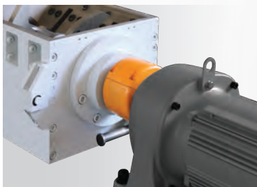
Gearmotor aligned with the rotor by interposed chain joint
